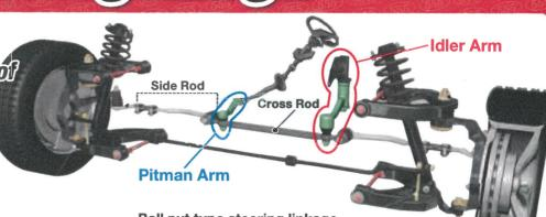
Ball nut type steering linkage
